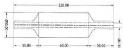
Polished thick-walled specimens Tests provide a through-wall strain gradient
